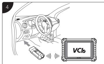
• When the MaxiVCI V200 is properly connected to the vehicle and the tablet, the VCI status button on the bottom bar of the screen will display a green badge with a check mark at the corner indicating the tablet is ready to start vehicle diagnosis.
